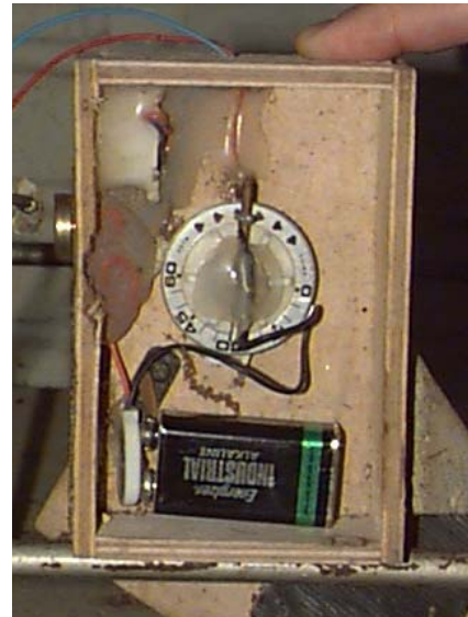
Battery attached to a timer switch
